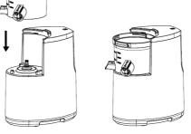
2.Align the screw shaft with the center of the juice bowl and insert it. After inserting the screw shaft to the bottom, rotate the screw counterclockwise, ensure that the screw is fully fastened to the main motor shaft in the main body.
