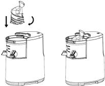
3.Install the filter screen, which should be vertically inserted into the feeding bowl according to the direction shown in the diagram and install in place.
