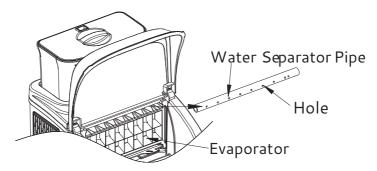
2. For both of the water tank and the big water reservoir, clean them with diluted detergent, warm water and a soft cloth. Then use the water to rinse the inside, and drain out the water from the draining port by unplugging the Water drainage cap on the bottom. It will help you keep the unit and ice-cube hygienicly, and also make the unit work normally.
